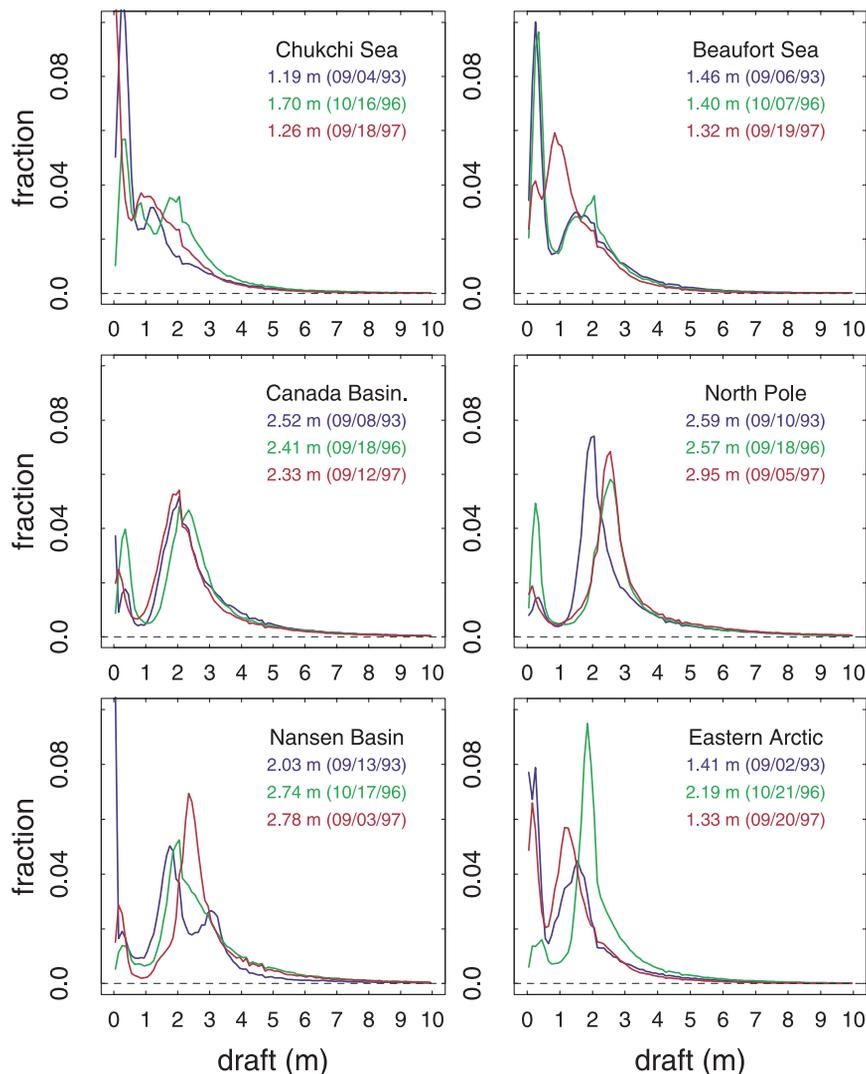
**Figure 3.** Regional ice draft distributions from the three SCICEX cruises in 1993, 1996, and 1997. The draft bin is 10 cm. Locations of the six areas are shown in Figure 1b. Average draft and date of each transect are also shown.
