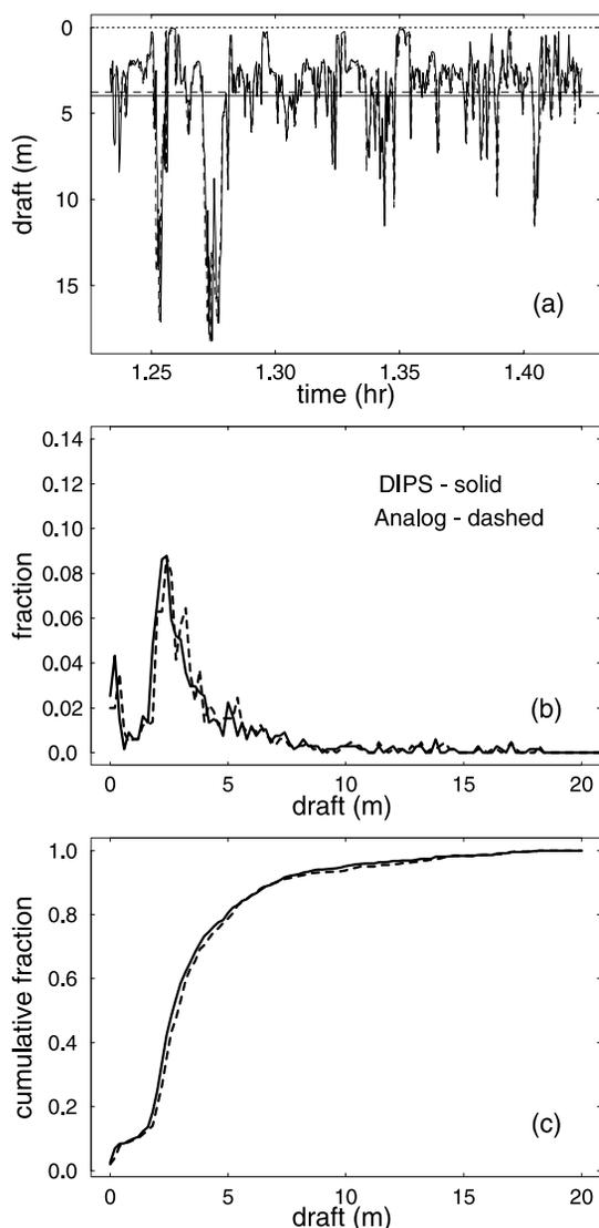
**Figure 2.** Ice draft comparison between analog chart and Digital Ice Profiling System for (a) profiles, (b) area fraction, and (c) cumulative distribution. The data were recorded along a 5-km SCICEX transect on 9 September 1997.
